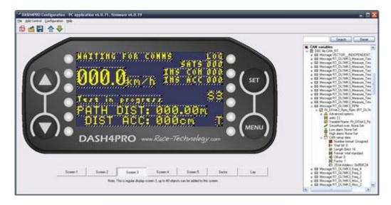
**New CAN output** commands help to integrate the DASH4PRO with third party equipment, with CAN messages being output to control other equipment. CAN commands can be output when the display screen is changed (useful for changing testing scenarios), or when a button (or combination of buttons) is pressed.
