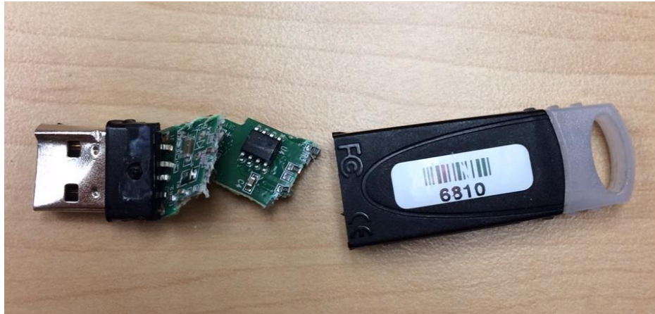
Figure 1. Example of destroyed USB key with serial number clearly shown
